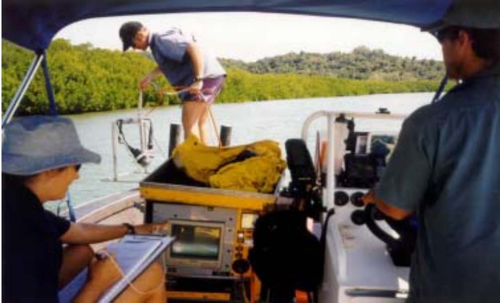
Plate 3 Underwater video camera used to survey seagrass, algae and other benthos in the Skardon River survey.
