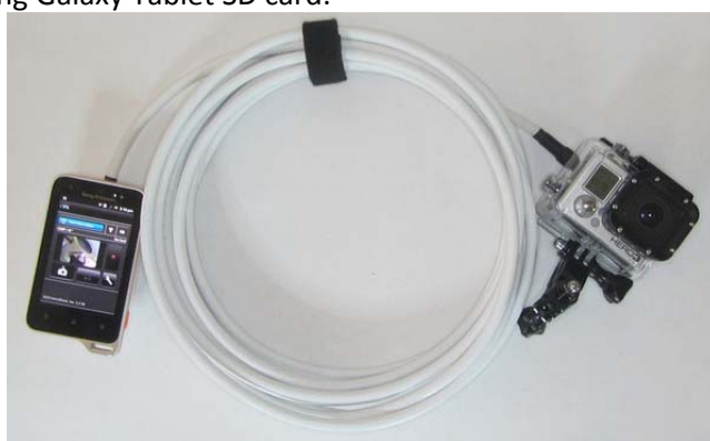
Figure 21. WiFi Extension Cable from cam-do.com, which extends the use of WiFi and Bluetooth control of GoPro® Hero3, cameras underwater. At the dry end, the WiFi extension interfaces wirelessly with any Android phone or tablet or iPhone or iPad. The interface can be attached to the back of the phone (in this image a Sony Xperia Active) using velcro or 3M double sided removable mounting squares.
