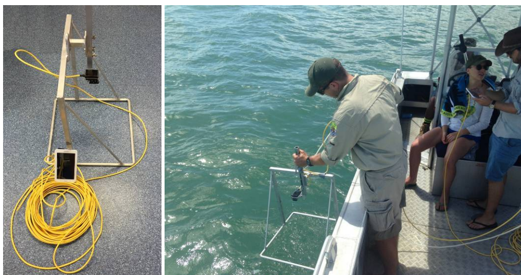
Figure 23. Drop camera assembly (left) and field deployment (right). Note GoPro® fixed at correct height to ensure 0.25m 2 quadrat is within field of view and focus, and Samsung Galaxy Tablet with App to control GoPro, view and record footage.
