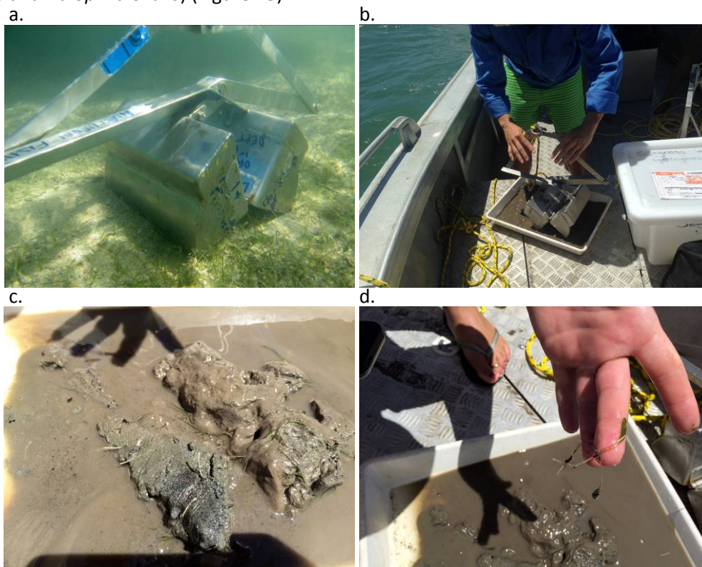
Figure 25. Van Veen grab, required to check sediment grain size and verify seagrass species: van Veen grab deployed (stock image) (a); sample released from grab (b); grab sample showing grain size (c); checking seagrass species (d).
