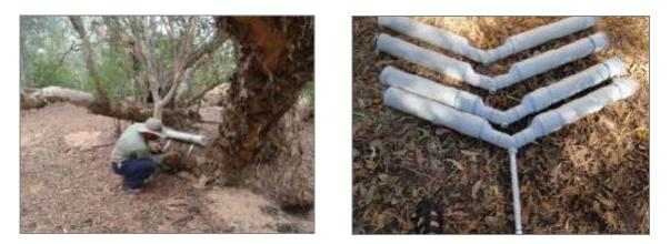
**Figure 8.** Integrated sampler being deployed (*left*) in the Hann River. A modified version of the integrated sampler (*right*) deployed for the first time as part of this study. This sampler is designed to collect a sequential deposit within the pipe protruding from the bottom of the sampler (i.e. layers of sediment that represent discrete events through the wet season). Source: Brooks *et al.* (2010).
