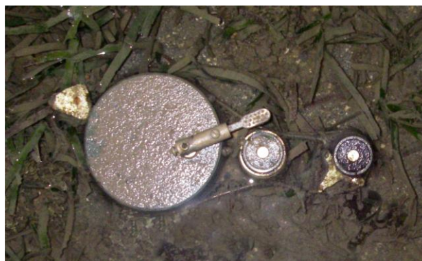
Autonomous submersible Odyssey™ photosynthetic irradiance loggers with (left) and without (right) a wiper unit at Cockle Bay
