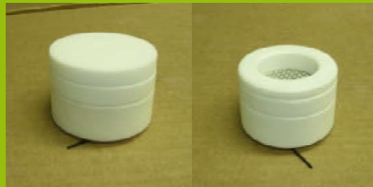
Empore Disk deployment device. Left - sealed with the transportation cap. Right - ready for deployment.
