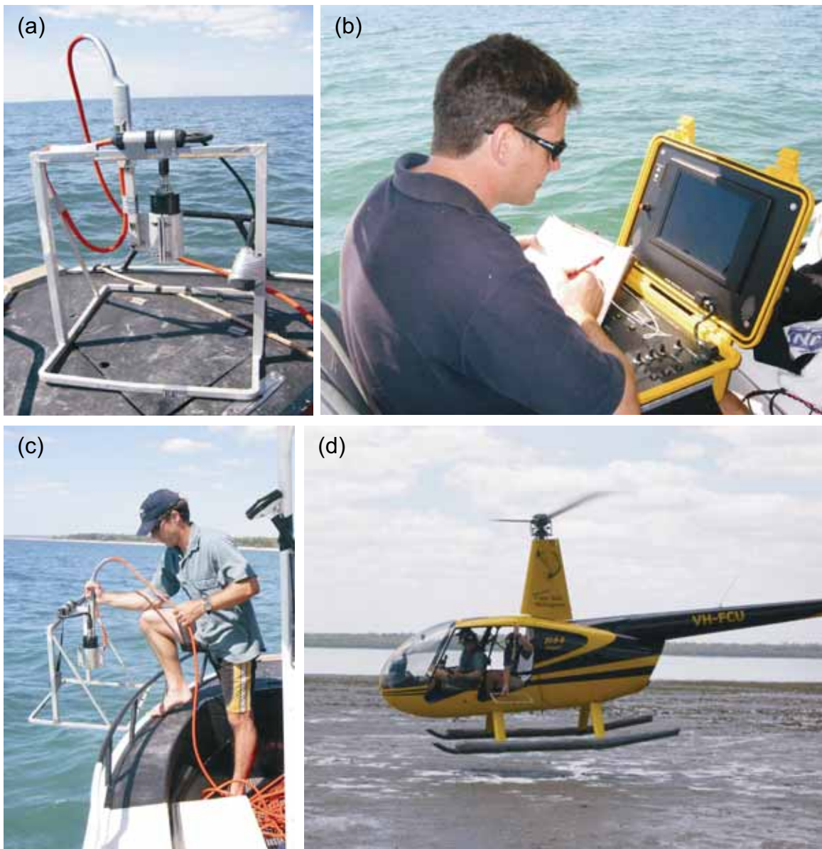
Plate 1 Seagrass monitoring techniques and equipment used at the Port of Weipa, 2000 to 2005: (a) underwater real-time video camera and frame (b) underwater video control panel and viewing screen (c) deploying underwater video camera from survey vessel (d) estimating above ground seagrass biomass from helicopter.
