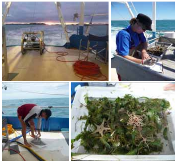
Plate 1. Offshore video sampling sled, Van Veen sediment grab and sorting benthic samples from the sled net
