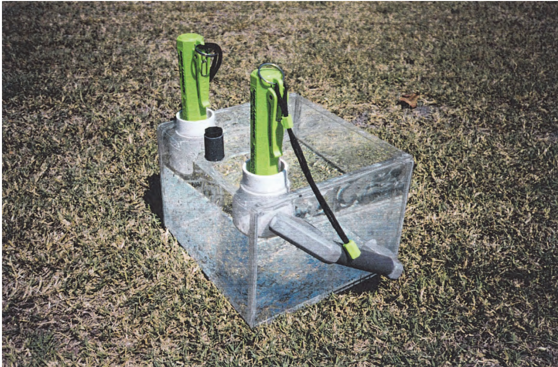
Figure 4. Illuminated underwater seagrass viewer used for conducting visual estimates of seagrass biomass in highly turbid waters.
